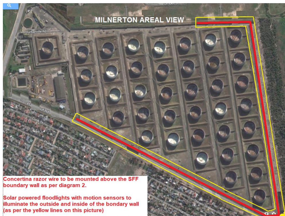
Diagram 2: setup of required concertina razor wire setup to be mounted via steel brackets above the SFF Milnerton boundary wall.
